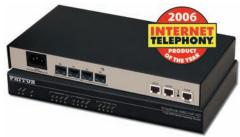
Providing a high-density seamless link between the circuitswitched telephone network and voice-over-IP, the SN4960 is ideal for PBX business trunking or corporate VoIP access. Offering up to four software configurable T1 /E1 /PRI interfaces the SN4960 connects to any switch, PBX and data network with up to 120 simultaneous calls using SIP, T1, E1 or PRI signaling. The dual gigabit Ethernet ports connect to the network for the highest throughput with its integrated QoS router. With
